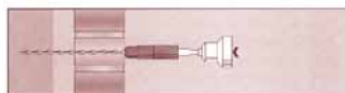
3 Drive in the small outer end to fully recessed below face of masonry and then make good.
